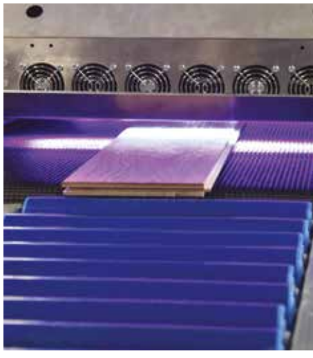
LED-CURING INDUSTRY UNIT INSTALLED ON THE RUBIO® MONOCOATER
